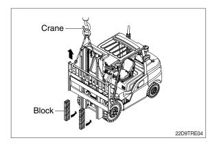
② While supporting lift chains, remove nuts and split pin from the anchor bolt.
