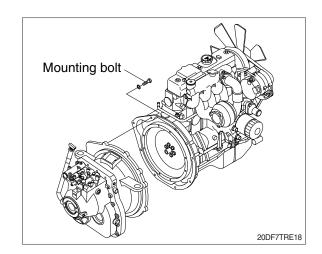
② Using a moving truck slowly pull out transmission assembly to the front.
