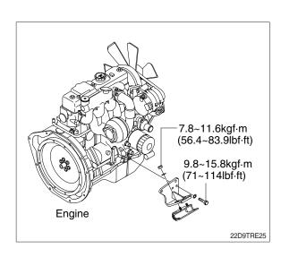
(3) Tightening torque of mounting bolt installing to torque converter housing.
